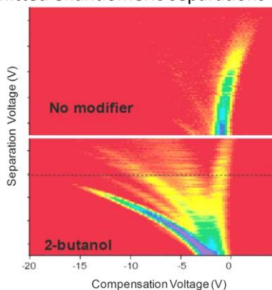
Figure 1. Effect of reagent gas (chemical modifier) on dispersion plot in DMS measurement of peptide.
