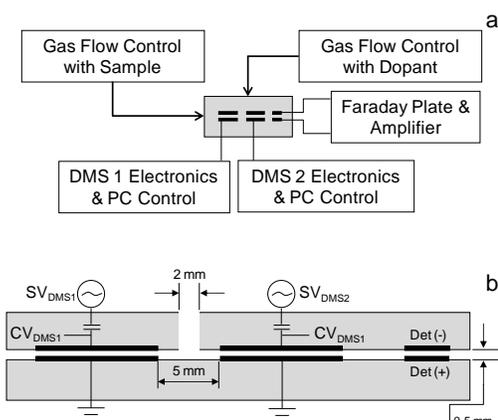
Figure 2. Schematics of (a) DMS/DMS system with (b) enlarge graphic of DMS/DMS analyzer with two stages: DMS1 and DMS2.
